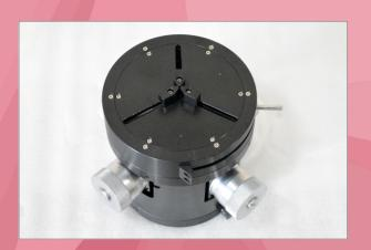
Self centering mechanism can help the object to place at center easily
